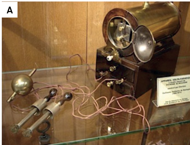
Figure 2. (A) The faradic voltage induction apparatus idealized by Duchenne. Musée d'histoire de la médecine, Paris . PM-F photograph. (B) A bas-relief medallion shows Duchenne using the apparatus and stimulating the forearm muscles of a patient lying in his bed 12 .
